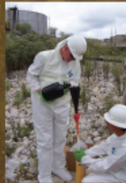
Pouring Fluorescein dye into well
