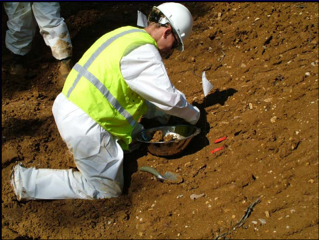
Verification samples taken on sidewalls
